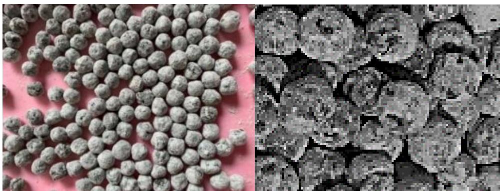
Gambar 1. Bentuk matriks urea enkapsulasi Figure 1. The form of encapsulated urea matrix
